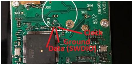
9. connect the ST Link pins to the respective pins on the radio. ST Links usually have female to female jumpers. I have found that sewing needles fit perfectly in the female jumper connector and this radio.
