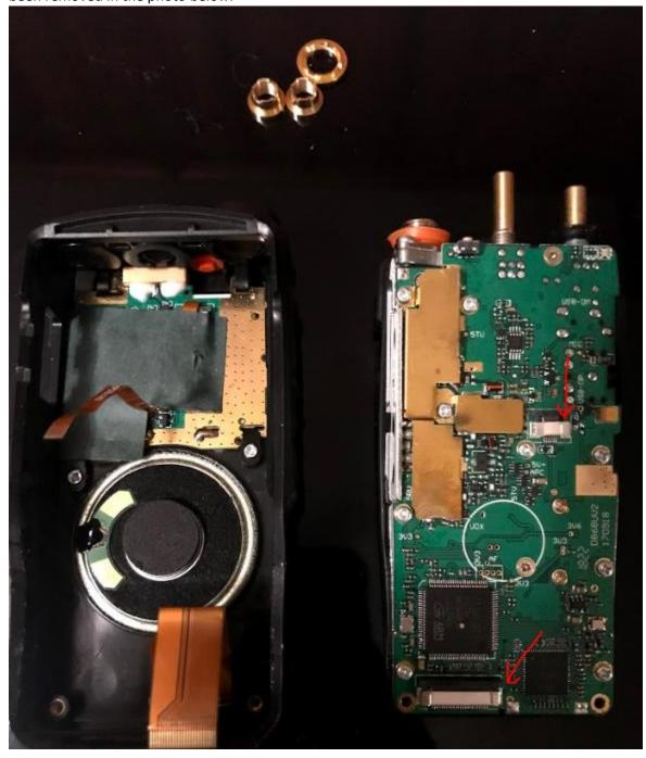
8. Locate the 3 programming pins that we will be using to update the radio.
