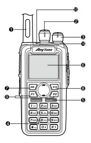
Press 7 (Menu) key to enter the menu, press very key to the Device Info and enter into the menu to check the hardware version.
